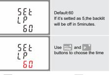
Press E to confirm the setting and press K to return to the main set up menu.
