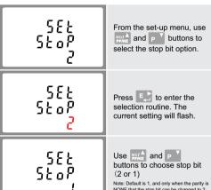
On completion of the entry procedure, press the setting and press  $\frac{V/A}{EEC}$  to return to the main set up menu.
